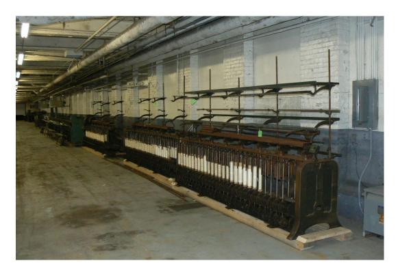
Figure 1 Spinning Frames in Storage
