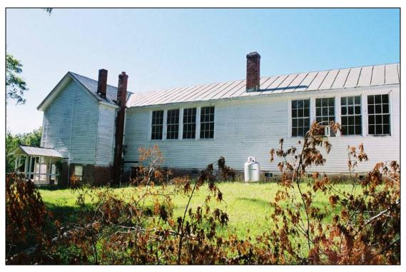
Plate 161. Castalia School: south elevation of classroom addition, with original banks of windows, at center; cafeteria at left
